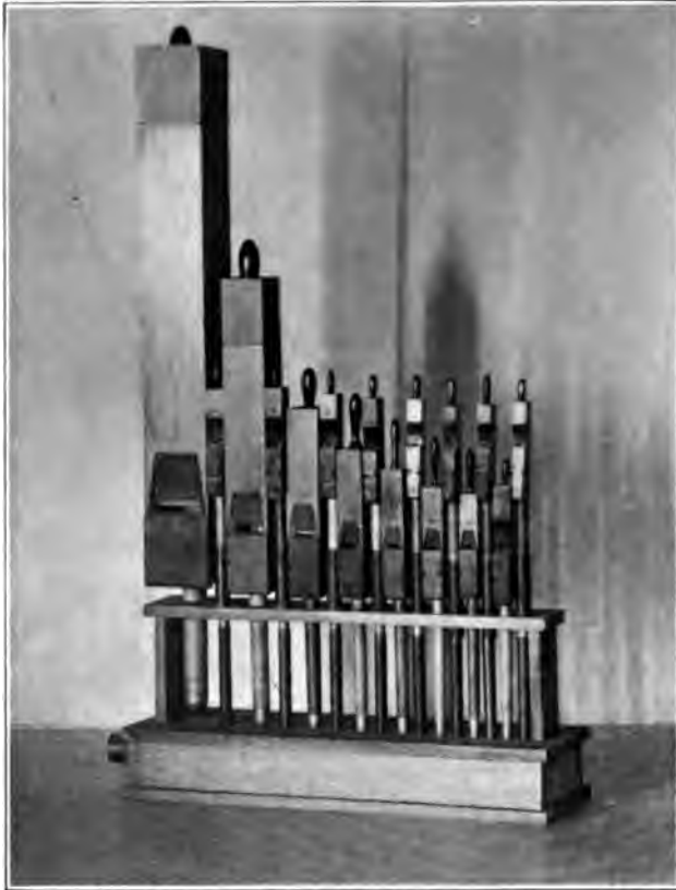
FIG. 180. Group of organ pipes, which, when sounded simultaneously, reproduce the vowel á in mat .
